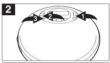
Within ten seconds, select the desired preset using the PRESET UP ▲ ① or DN ▼ ② button to set the memory. Press the PROG. button ③ to confirm.
