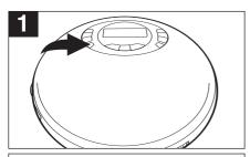
While in the Stop mode, press the PROG. button. The track number will blink and "P-01" will appear in the display.
