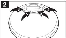
Select the first letter of the file you would like to listen to using the MODE/◀ ❶ and/or RESUME/▶ ❷ buttons. Press the PRESET DN ▼ button ❸ to access the lower letters or PRESET UP ▲ button ❹ to access the higher letters.
