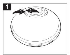
During playback, depress and hold either the Skip/TUNING DN IM ① or UP IM ② button to move the player forward or backward within a track to locate a specific musical passage. The player will move forward or backward at high speed as long as the buttons are depressed. When you release the Skip/TUNING DN IM ① or UP IM ② button, normal playback will resume.
