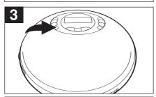
Press the PROG. button to memorize the track. Repeat steps 2 and 3 to program additional tracks up to a maximum of 24 tracks.
